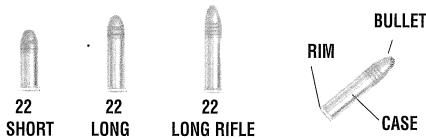
PICTURE 2 This picture shows the main parts of the ammunition. 22 CALIBER CARTRIDGE
