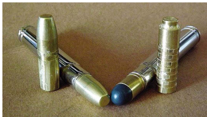
Bullets dislodged after penetrating four feet of hardwood. Left, Nosler noted in article; right, Woodleigh, after shedding its rounded cap, used to facilitate feeding from magazine to chamber.
