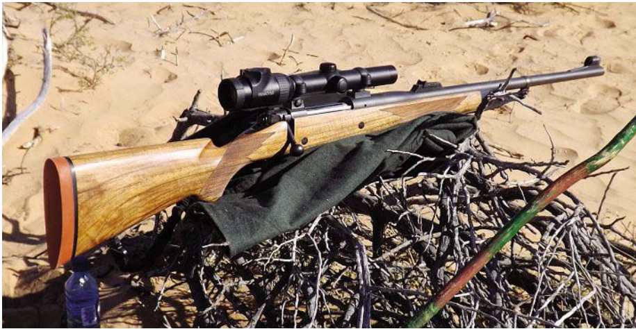
Above: The Kimber Caprivi comes in .375H&H, .416 Remington Magnum and .458 Lott. The author chose the .416 for both its near and far performance. The author's rifle has dual opposed locking lugs; full length claw extractor; three position wing safety; hinged floor plate; folding three leaf open sight; hooded front sight on 24-inch barrel; straight comb AA French walnut stock for recoil management; front barrel band sling swivel; Decelerator recoil pad; hand checkering. The author's original Swarovski 1x-6x was replaced with a Swarovski 2x-12x for both close and longer-range shooting.
